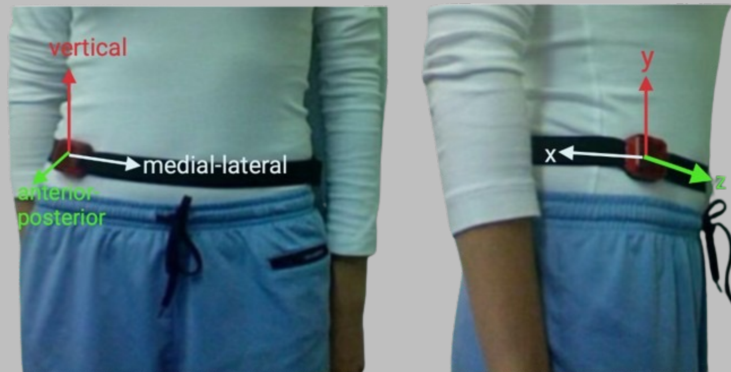
Figure 1: Participant wearing an ActiGraph GT3x accelerometer, depicted with a display image pictograph, illustrating the three-axis visual representation.
